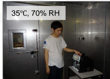
High temperature and humidity testing
