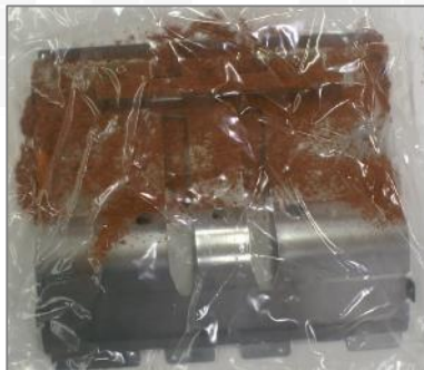
Dust ingress testing
