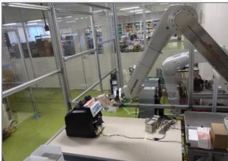
Endurance test by robot
